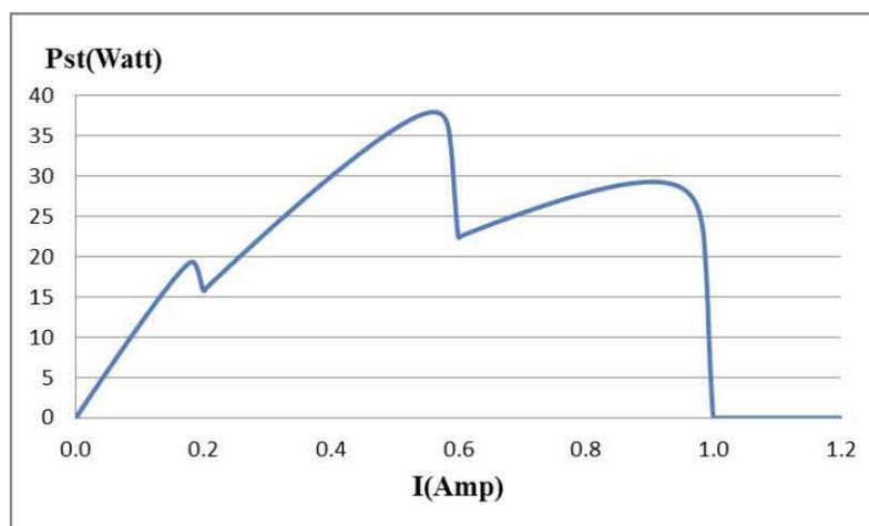
**Figure 1.** P-I curve of a string with 3 PV panels receiving 1000, 600 and 200W/m<sup>2</sup> irradiances (left) and PV string with distributed DC/DC converter (right).
